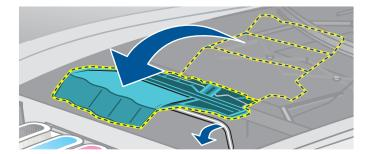
3 Pull the latch up and back to uncover the printheads.
